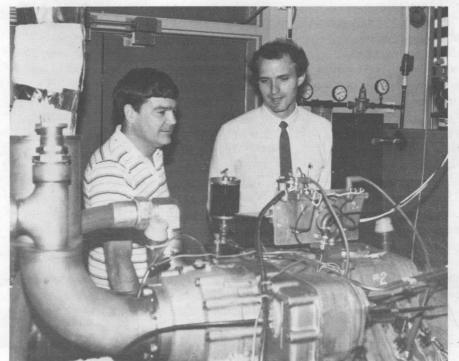
JOHN DEERE's prototype 750-horsepower rotary engine (foreground) got a workout while at CRF last year. Pete Witze (DMTS, 8362, left) and Philip Dimpelfeld (DOE Industrial Fellow from John Deere's Rotary Engine Division) ran the large Wankel-type rotary engine through its paces, measuring in-cylinder air velocities and turbulence to verify a John Deere multidimensional computer model.
